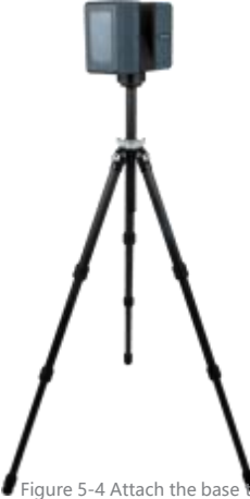
Figure 5-4 Attach the base to a tripod
