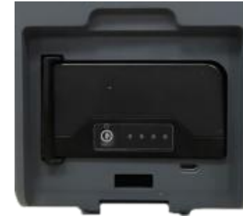
Figure 5-6: Insert the U disk
