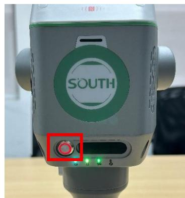
3. Description of Indicator Lights, from left to right in sequence are **Slam light**, **Data light**, **Satellite light**, **Power light**.
