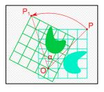
orientation, P1 is real back sight, after reduction, all points collect in blue gird will turn to real coordinates shows at green gird. we need to get the P1 real coordinate before process reduction.
