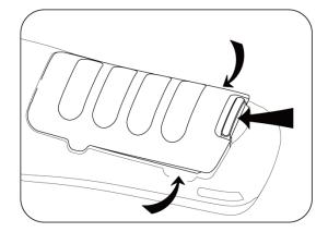
Push the battery release and mount clear the Push the battery release toward the top of battery to terminal and gently release it.
