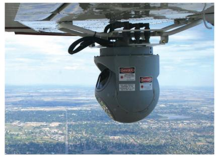
*Cameras mounted on aircraft require special stabilization to create clear images or motion pictures, surveillance, and other applications. The KVH DSP-3000 is an essential part of many of these systems.*
